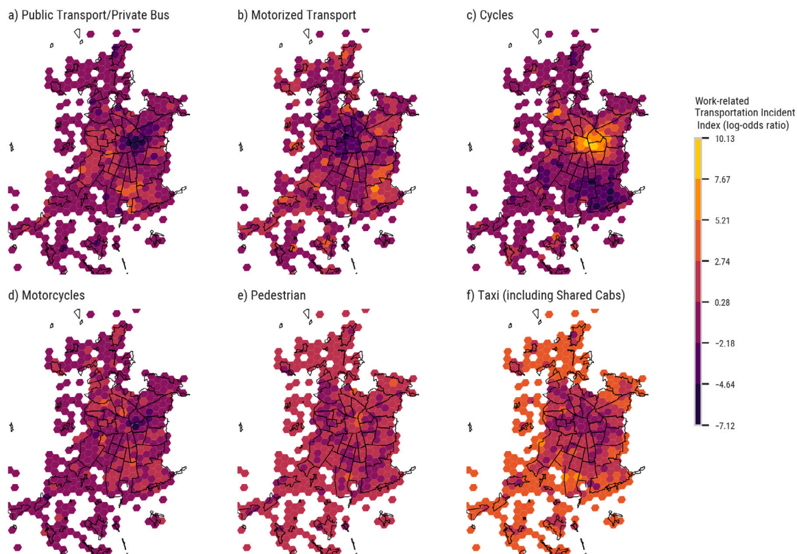
Fig. 7. Spatial associations with mode of transportation in each incident with cells from the H3 grid system. The association is defined as a log-odds ratio with an uninformative Dirichlet prior (Monroe et al., 2008). Each mode of transportation has its own map: (a) Public Transportation and Private Buses; (b) Motorized Transport (private cars and other vehicles with four wheels); (c) Cycles (including bikes and scooters); (d) Motorcycles; (e) Pedestrian; and (f) Taxi, including shared cabs, which are used predominantly in the south of the city. Positive log-odds ratios, depicted in shades of orange, signify areas where incidents in the respective mode are more prevalent than expected. Conversely, negative ratios, depicted in shades of purple, indicate fewer incidents than anticipated.
